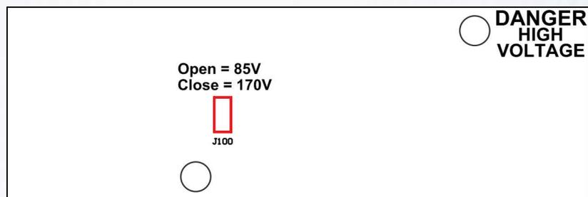
If the jumper is open detection level is 85VAC, if it is close, detection level is 170VAC.
