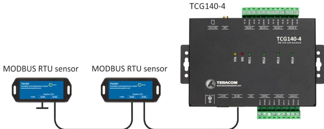
To maintain signal integrity, it is essential to use 120-ohm line terminators at both ends of the RS-485 bus. The TCG140-4 includes one terminator and should be installed at one end of the line, leaving the other end for the user to terminate.
