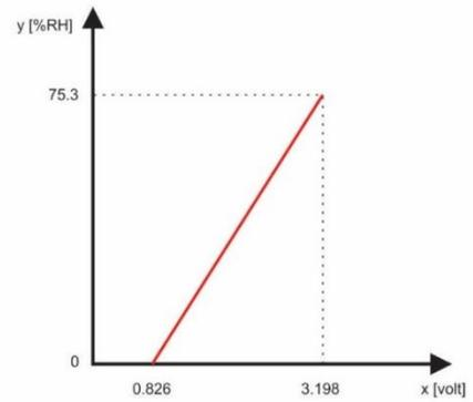
The sensor outputs raw voltage values, but our goal is to convert these into corresponding relative humidity (RH) values. To achieve this, we use a multiplier and an offset. These parameters enable us to calculate the relative humidity for any voltage within the sensor's operational range.
