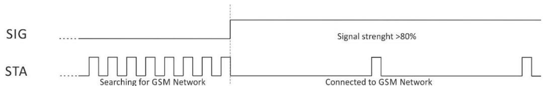
If there are GSM and 4G/3G/2G connections available, the STA indicator flashes twice for 200 milliseconds within a 2-second period.
