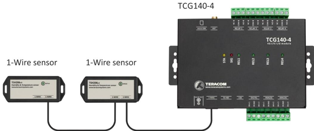
It is strongly recommended to use only UTP/FTP cables for the 1-Wire interface and to keep the total cable length within 30 meters. While functionality has been observed at longer distances, error-free operation cannot be guaranteed beyond the specified limit.
