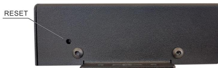
Factory default settings can also be restored from the SETUP -> System page by clicking the "Reset to default" button.
