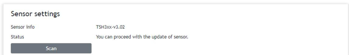
The firmware update tool operates using the current MODBUS RTU communication parameters. To prevent communication conflicts, it is recommended to configure both the TCG140-4 device and the sensor with the factory default MODBUS RTU communication parameters. This practice ensures seamless operation. The default communication parameters for the TCG140-4 are outlined in Section 9.2.1.
